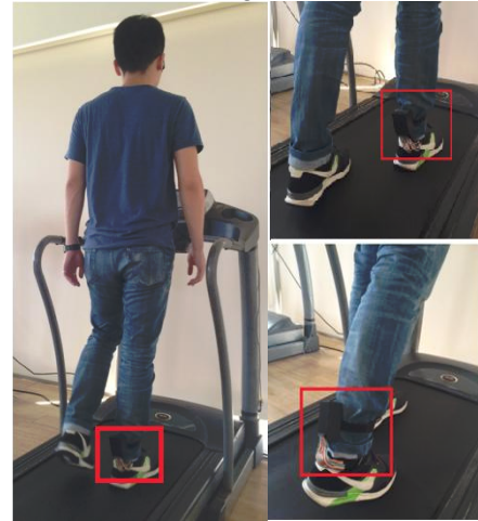
Fig. 3. Subject walks on the treadmill with 4 km / hr to simulate walking scenario.
