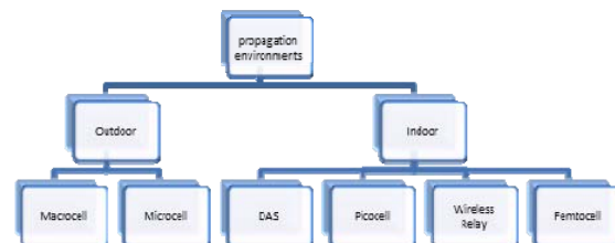
Figure 3. Type of Base Station According to Propagation Environment
