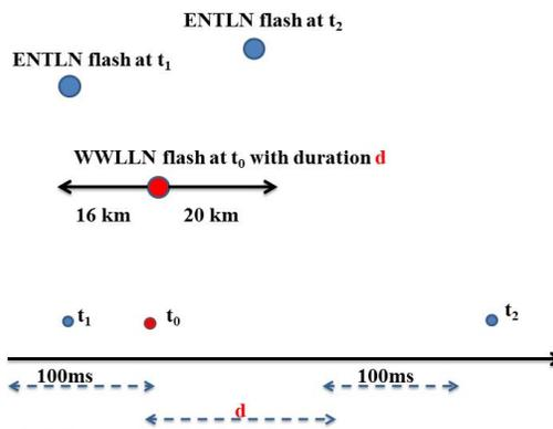
Fig. 2. An example of identifying coincident flash between two networks.
