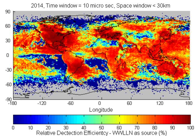
Fig. 6. ENTLN's Detection Efficiency in 2014 within 10  $\mu$ s in time window and distances between station < 30 km.
