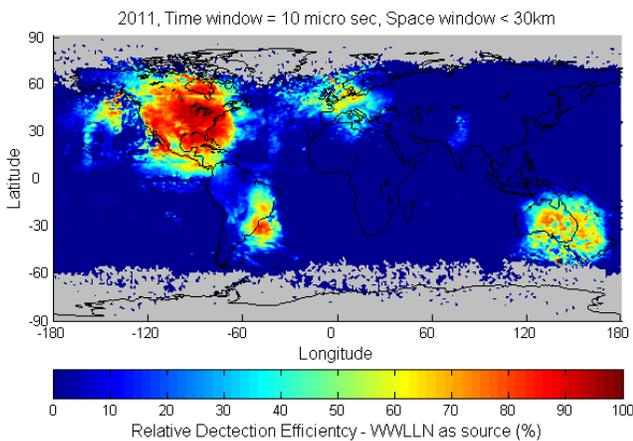
Fig. 4. ENTLN's Detection Efficiency in 2011 within 10  $\mu$ s in time window and distances between station < 30 km.
