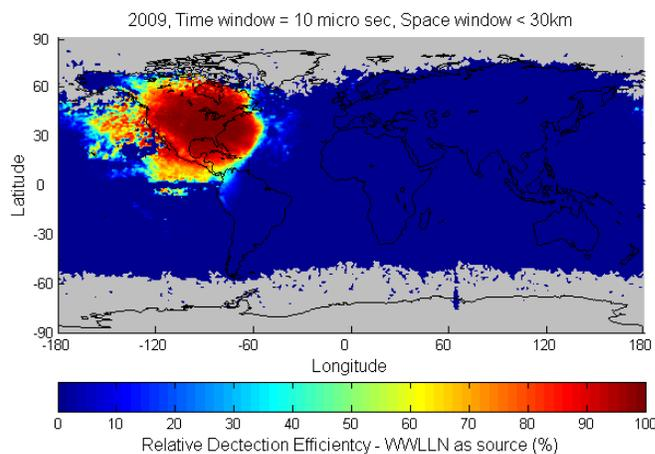
Fig. 3. ENTLN's Detection Efficiency in 2009 within 10  $\mu$ s in time window and distances between station < 30 km.
