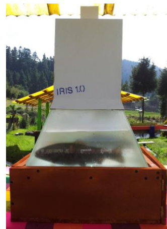
Figure 4. Functional prototype used within our measuring system. This prototype includes an illumination source, a pyramidal canalisation compartment and a 2D camera.
