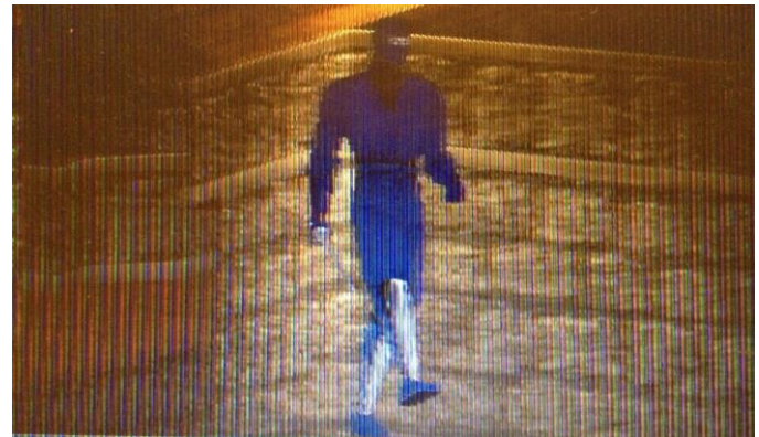
Fig. 7. An integrated image as it is seen using a primitive microlenses array.
