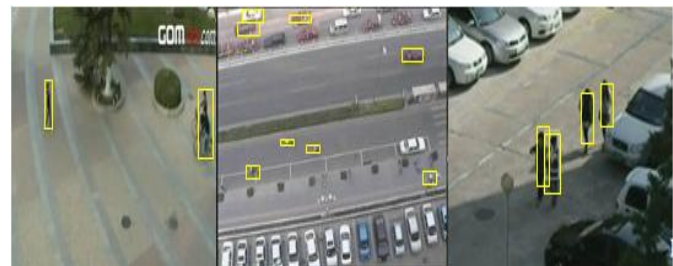
Fig. 6. Results of object tracking using SIFT and Kalman Filter.
