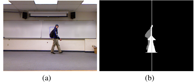
Fig. 5: (a) A person is tracked along with his backpack. A blue square is drawn around the backpack. (b) The internal representation of each blob in the backpack module. The dark grey vertical line represents the computed symmetry axis, the white regions are considered symmetric, and the grey regions are considered asymmetric.
