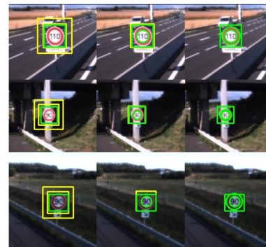
Fig. 8: Some focus examples for a road sign. In yellow it is the detection zone and in green it is the parts already detected. In the first column, as the detector of red returns really unaccurate zone, the detection zone for circle is bigger than the red zone found. In the second column, the detection for the last circle (the big one) is smaller than in the first column : as the little circle has been detected and its detector is more accurate, the zone has been reduced. The last column shows all parts found.
