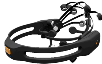
Figure 1. EEG Emotiv EPOC Device.
