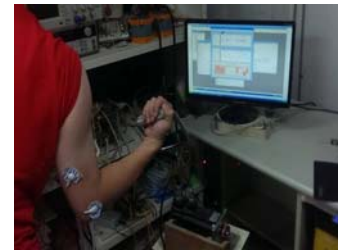
Fig. 4. The practical system of ASTM with EMG sensors.
