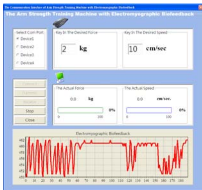
Fig. 2. The test for force 2 kg-cm, speed 10 cm/sec and EMG
