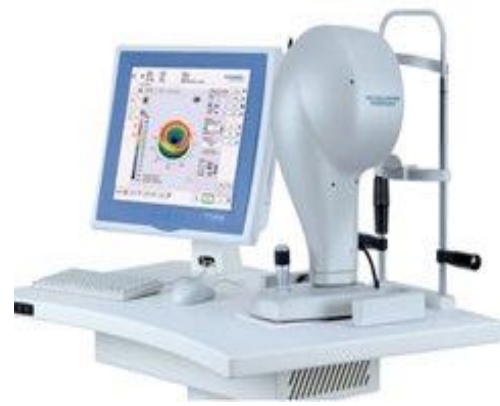
Fig. 3. Scheimpflug Camera and Placido Disc Combination [13]
