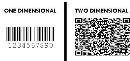
Fig. 1 Differences between one and two dimensional code
