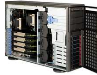
Fig. 1: Four NVIDIA GPUs installed in a workstation.
