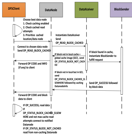
Fig. 3: DFSClient and DataNode Interaction Sequence Diagram
