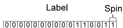
Figure 3: Bit-packing used to store a cell's spin and label in the same 16-bit unsigned short int. This cell is 'alive' and has the label 25.
