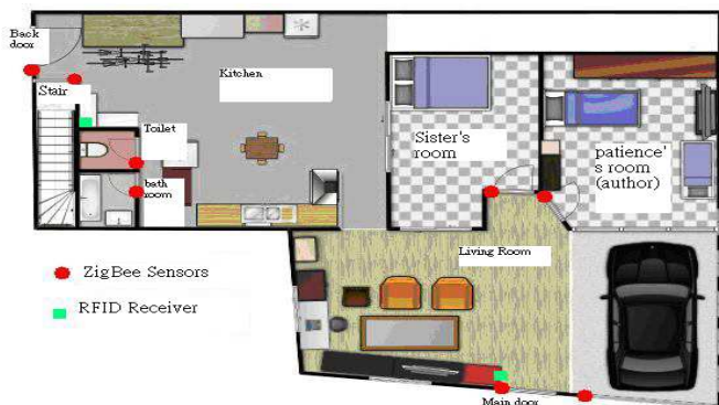
Figure 1: The schema of house and two devices installed
