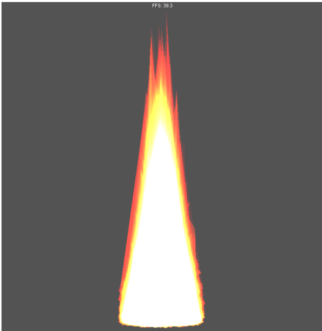
Figure 7: A simulation of the 128x128 fire particle system (16384 particles) rendered using VBOs and GL TRIANGLES
