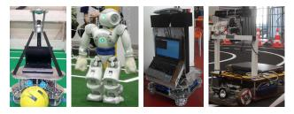
Fig. 2: Robotic platforms used in this work. From left to right, CAMBADA (RoboCup Middle Size league robotic soccer), NAO (RoboCup Standard Platform League soccer robot), CAMBADA@HOME (service robot for elderly and disabled people support - under test on RoboCup @HOME league) and autonomous driving.
