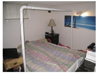
Fig. 12: Measurement Setup for human trial measurements. When the trials are taking place all lights are shut off and the room is darker.
