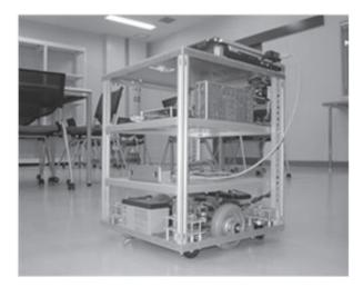
Fig. 9. Stereo video camera and robot platform.
