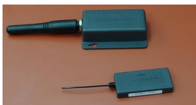
Figura 4. RFID reader and active tag
