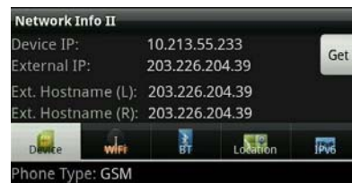
Fig. 6. Check IP address assigned to the smart-phone via Network Info II.
