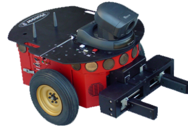
Fig. 5: A typical prototype of Pioneer 2-DX robot with gripper.
