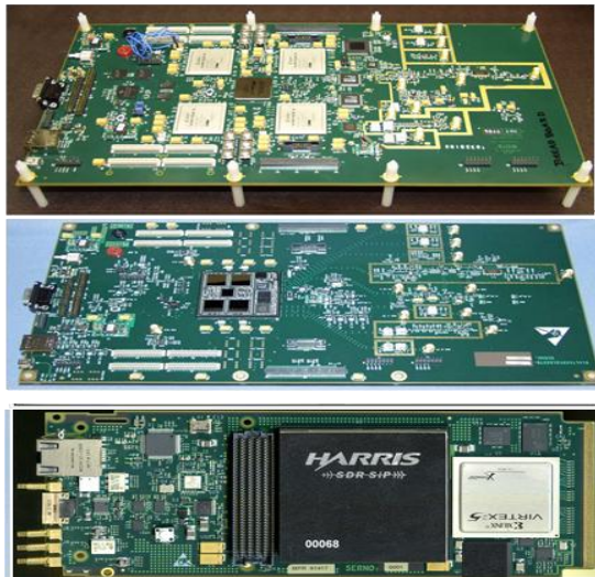
Figure 2-3: Evolution of the SiP-100 multi-mission platform from packaged parts development card (top), prototype SiP development card (center), and SiP deployment in an integrated \mu TCA implementation (bottom).
