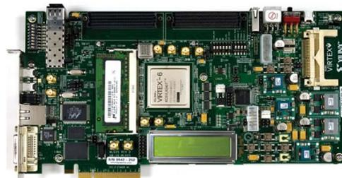
Figure 1: ML605: Xilinx Virtex 6 development board
