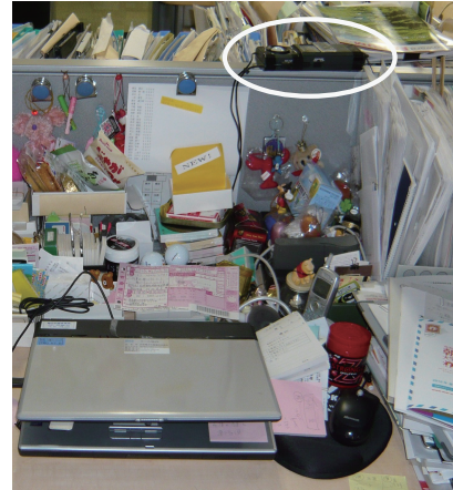
Fig. 3. A situation prohibiting the placement of an illuminance sensor on the workplane (example)
