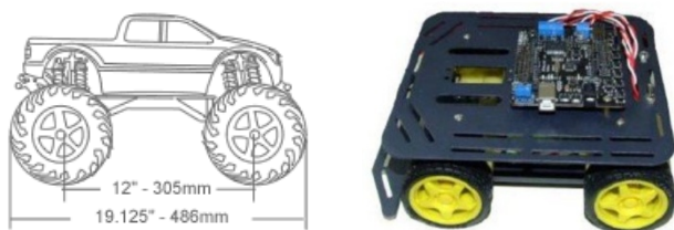
Figure 1: MOSES Drivetrain (Traxxas left, DFRobot right)
