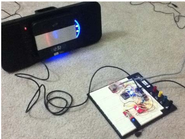
Fig 9 An mbed-based internet radio built using Ethernet, USB, stereo audio jack, and MP3 audio decoder breakout boards.
