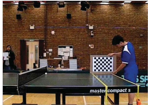
Figure 4 A double-sided checker board used for calibration
