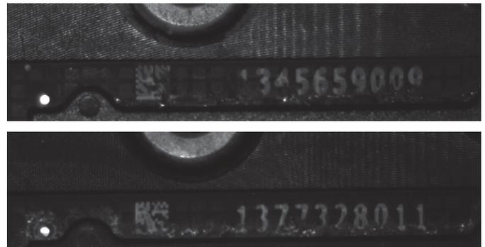
Fig. 2. PCBs with evident residual dirt over characters.
