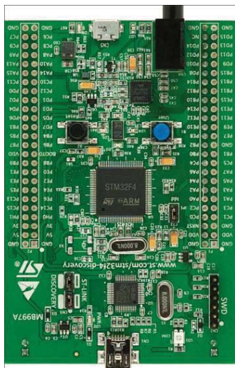
Figure 3: The STM32F4-Discovery Board used for execution time and power measurement.
