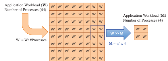
Fig. 8: Emulating the computation time of a process changing the application workload
