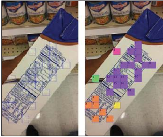
Figure 3. Square tiles with pronounced changes (left); Tile clusters found by DFS (right)
