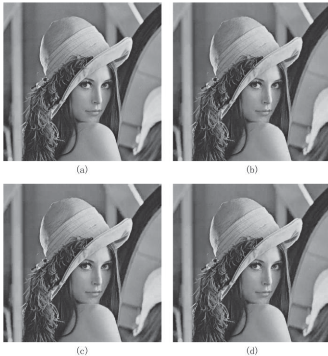
Fig.2 Original image and reconstructed images; (a) Original image ('Lena'); (b) reconstructed image by random sampling algorithm; (c) reconstructed image by average separation algorithm; (d) reconstructed image by mean/variance classification algorithm.
