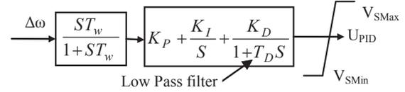
Figure 1. Structure of PID stabilizer
