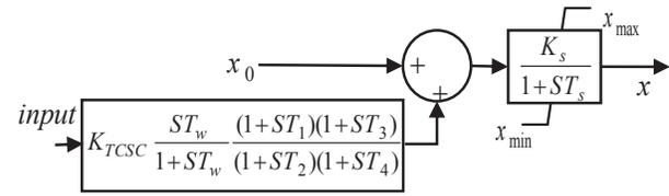
Figure 2. structure of TCSC based controller
