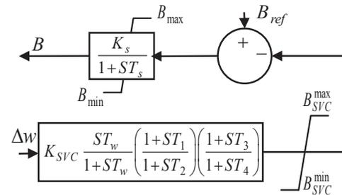
Figure 3. structure of SVC based controller
