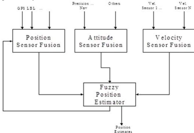
Figure 8 - High-Level Fusion Architecture for PNT Estimation
