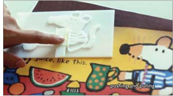
Figure 1. An example of a 3D printed page from a tactile storybook (image courtesy of [25])
