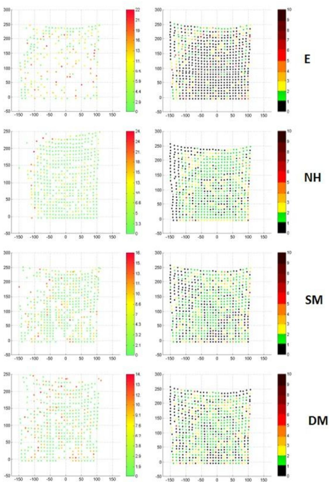
**Figure 2.**Distance map [mm] (left column) and correspondence map [number of units] (right column) for different modifications of ICP computing correspondence: Euclidean distance (E), normal shooting with initial rigid registration (NH), static marker vectors (SM), dynamic marker vectors (DM).
