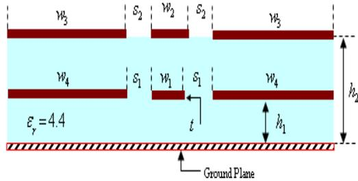
Fig. 2. Cross section of multilayer CPW broadside coupled-line balun.
