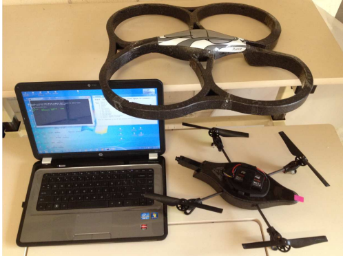
Fig. 1: Parrot ARDrone 1.0 with indoor hull and a laptop as the ground station.
