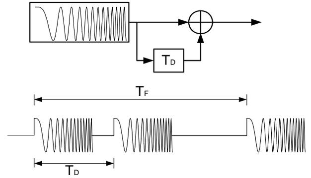
Figure 1. Signal scheme of TR-FMCW-UWB radar
