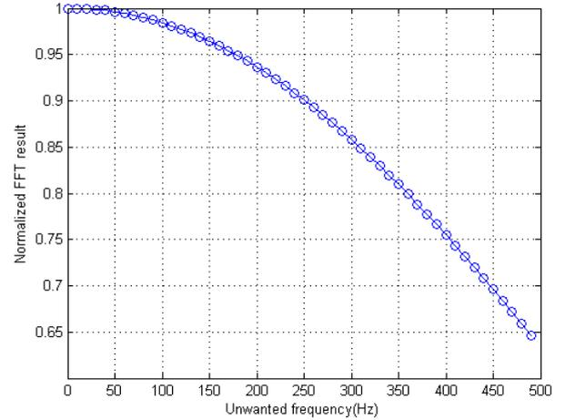
Figure 3. FFT results with effects of unwanted frequency
