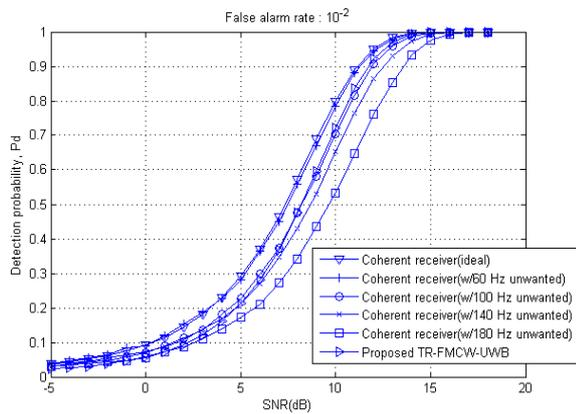
Figure 4. Detection probability of the proposed radar compared to that of the coherent receiver according to unwanted frequency
