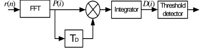
Figure 2. Block diagram of TR-FMCW-UWB radar receiver
