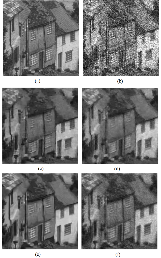
Fig. 6: (a) Part of the original Image Goldhill at peak intensity 20. (b) Poisson noise corrupted image. (c) Image denoised with overcomplete SURE-LET [14] and the proposed inversion. (d) Image denoised with PURE-LET [8]. (e) Image denoised with BM3D and their unbiased inversion [5]. (f) Image denoised with the proposed method CMWT-IAT.
