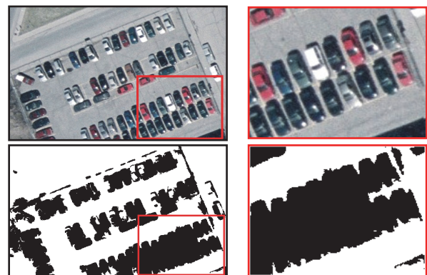
Fig. 7 (a) Multi-scale SLIC is applied on entire image (top left) and (b) on a sub-image (top right). Their salient regions are respectively given by (c) and (d), the bottom-left and the bottom right images. Cropping the image has no effect since a pixel-based decision rule is used, Eq.4.
