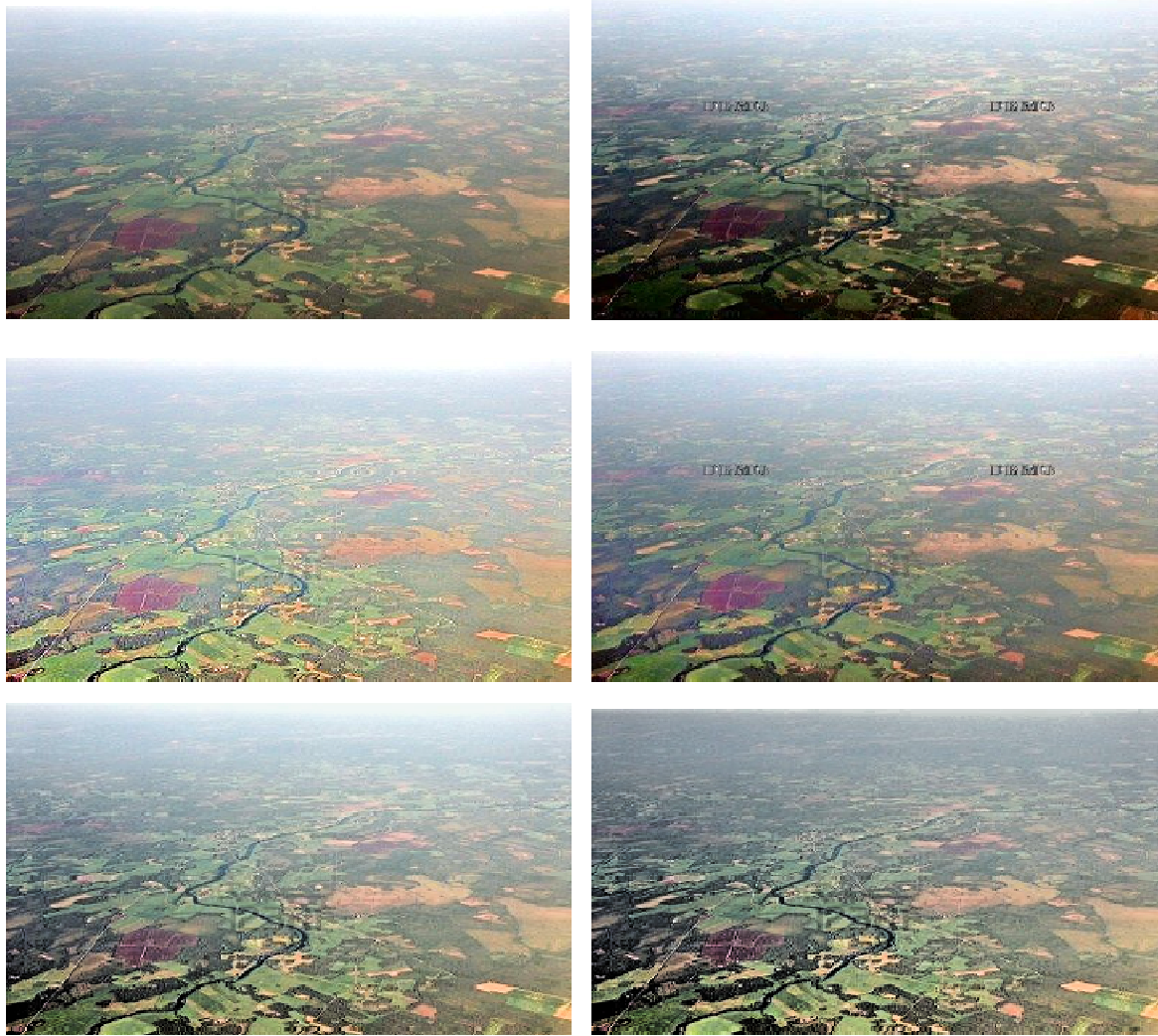
Figure 5. Comparisons: (top-left) Original; (top-right) Histogram equalization; (middle-left) IRME; (middle-right) MSR; (bottom-left) AINDANE; (bottom-right) METNUD.
