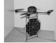
Figure 10: Helicopter with a vertical solar panel underneath [7]
