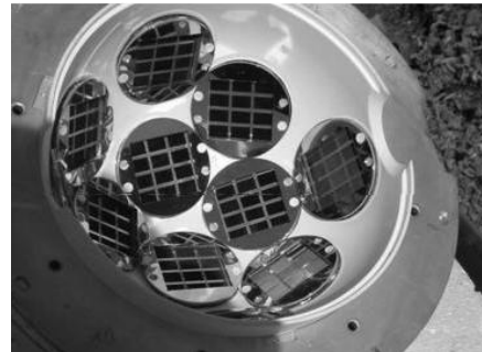
Figure 8: The interior of the PowerSphere (one of the two hemispheres) [1]
