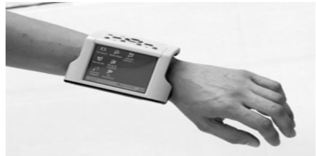
Fig 3.5.1 Novel TMS320 DSP based Multipara System
