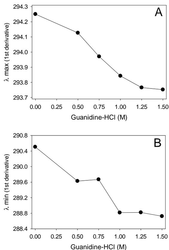
**Figure 3: First derivative maxima and minima as a function of chaotropic agent, GdnHCl.** First derivatives were initially computed for the downslope of the UV spectra; then the wavelengths representing zeniths (A) and nadirs (B) ( $\lambda$  max and  $\lambda$  min, respectively) were plotted as a function of GdnHCl concentration.
